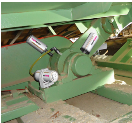
The bearings of a vibration channel are lubricated continuously by three lubricators.
