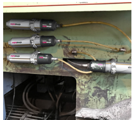
Thanks to the simalube IMPULSE pressure booster, the lubrication points at the winder (bearings, guide bushes and interlocks) can be installed remotely and supplied with lubricant via a hose installation.
