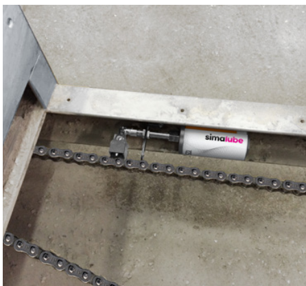
If there are space constraints, simalube can also be installed at an angle.
